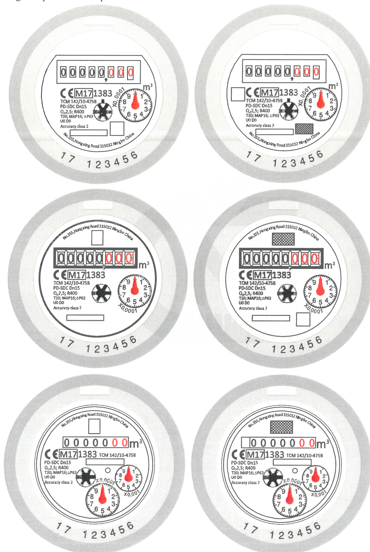
Figure 12: The dial plates of the water meter type PD-SDC (E8). Variant with inductive pointer or magnetic pointer is also possible.
