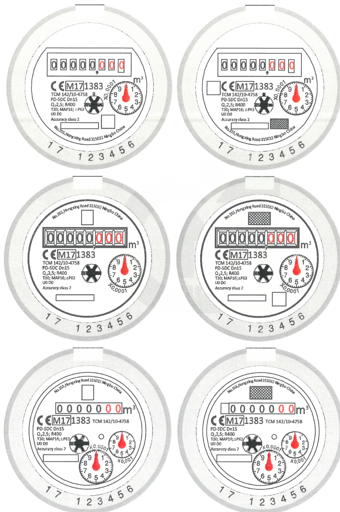
Figure 9: The dial plates of the water meter type PD-SDC (E4). Variant with inductive pointer or magnetic pointer is also possible.
